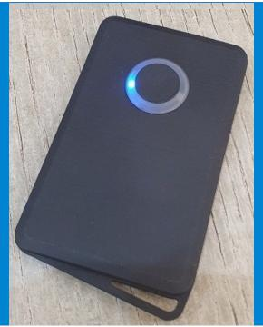
**UHF Scanner RE40** is a powerful RFID reader, capable of reading UHF tags and transmitting the acquired data to any device equipped with a Bluetooth interface, including Android or iOS smartphones and tablets.
