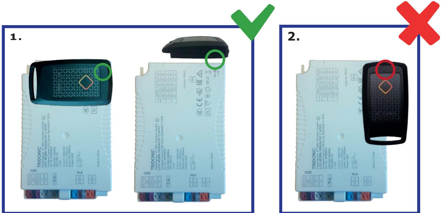
As regards the optimal reading of the LED driver, NFC Scanner must be positioned “edge reading” over the NFC area of LED driver or sideways as shown in figure 1.
