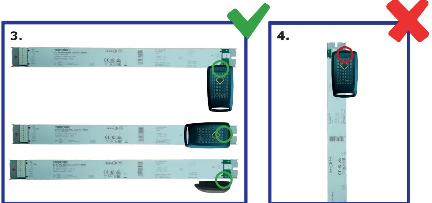
As regards the optimal reading of the LED drivers, NFC Scanner must be positioned at right angles to the LED driver, or in “edge reading”, or sideways from the NFC area logo as shown in figure 3.
