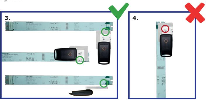
For optimal reading of LED drivers using NFC Passive Repeater, the reader must be positioned at right angles to the LED driver, or in "edge reading" over the NFC area of LED driver, in correspondence with "Focus 2" on the label, or sideways from the NFC area logo, as shown in **figure 3**.
