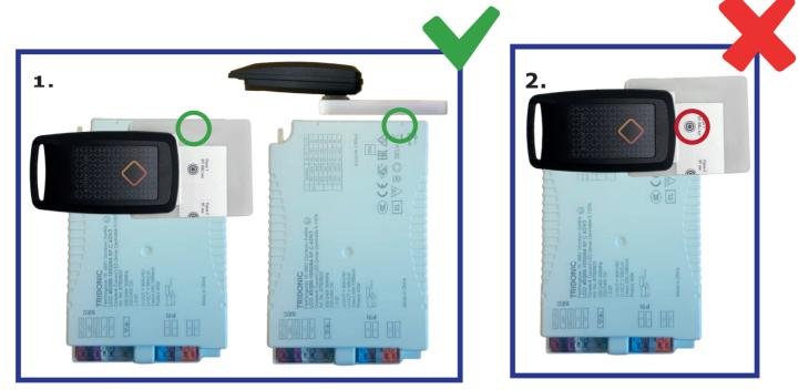
For optimal reading of LED drivers using NFC Passive Repeater, the reader must be positioned in "edge reading" over the NFC area of LED driver, in correspondence with "Focus 2" on the label, or sideways from the NFC area logo, as shown in **figure 1**.
