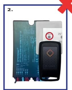
For optimal reading of OT LED drivers using NFC Passive Repeater, the reader must be positioned in "edge reading" over the NFC area of LED driver, in correspondence with "Focus 2" on the label, or sideways from the NFC area logo, as shown in figure 1.
