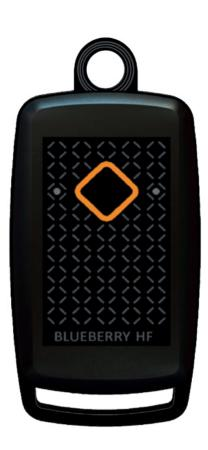
BlueBerry HS HF MS15 is a mobile mini RFID reader, shaped like a keychain, capable of reading HF tags and transmitting the acquired data to any device equipped with a Bluetooth® radio interface.
