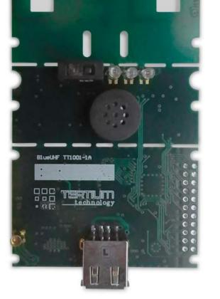
The BlueRFID UHF electronic card is a small desktop RFID reader, able to read and write UHF tags and transmitting the acquired data to any device with a USB interface.
