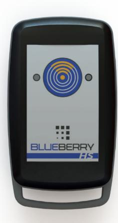
BlueBerry HS UHF is a mobile mini RFID reader, shaped like a keychain, capable of reading UHF tags and transmitting the acquired data to any device equipped with a Bluetooth® radio interface.
